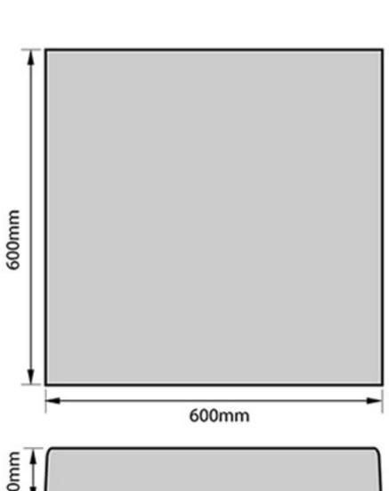
The **type 2** plinths are manufactured in either a dense concrete or a lightweight concrete.
